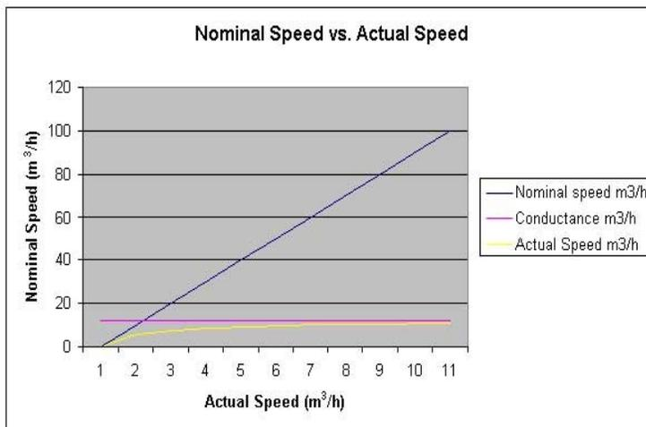
Using pumps that are too large is not only wasteful but may be dangerous as the larger suction capacity during initial pump-down causes an accelerated evaporation of moisture inside the system, causing freezing inside
