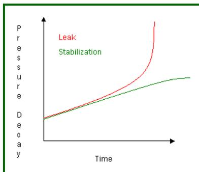
In profiling you are looking for the "sweet spot", so the target leak rate can be zeroed in by adding 50% of the actual leak rate at the time of the test's conclusion.
