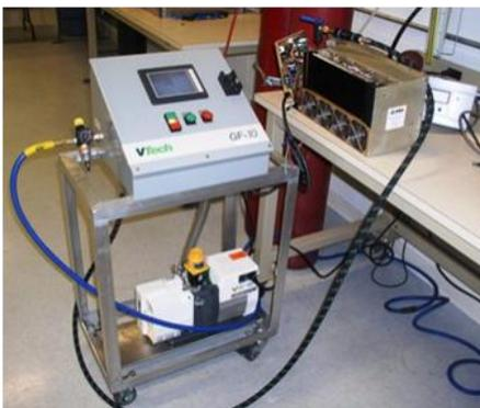
If Pressure Decay is not required or if it is handled by an existing system, then the [VTech Gas Fill Plus](#) can be used to evacuate and fill the gas only, and utilize a customer-supplied leak detector such as this bench-type configuration with the Gas Fill Plus working alongside the Hydrogen sniffing unit.
