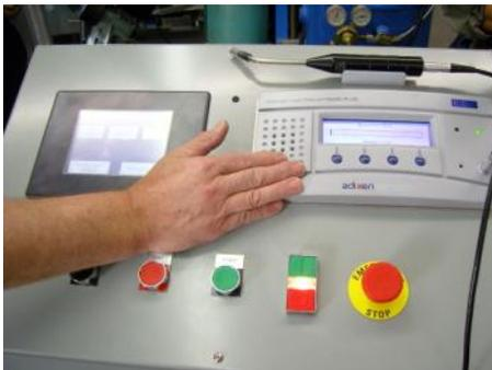
The [VTech 75 Multifunction Leak Detection System](#) combines evacuation, with a Venturi vacuum generator or optional vacuum pump, and precision tracer gas filling for manual sniffing leak detectors in either an integrated Hydrogen Detector or Standalone Helium Tester. The system also includes a preliminary pressure decay leak test, to prevent gross leaks from wasting valuable time--and tracer gas, in the fine leak detection process.
