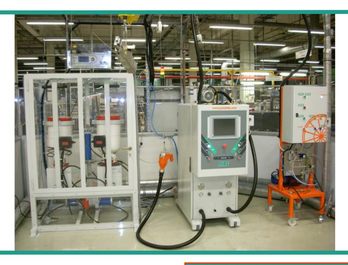
The VTech MRC-HC Automatic Evacuation and Refrigerant Charging System is designed for safely and accurately charging HC refrigerants and blends (e.g. R290, R600a, R170, R32) in a production environment. The system also performs an automatic vacuum cycle and a vacuum decay leak test, prior to refrigerant charging.
