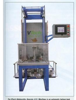
detector for testing refrigeration components and complete refrigeration units, even in the presence of polyurethane foam. It detects helium leaks as small as 0.1 oz of R-134a per year. It requires just 10% helium concen-
