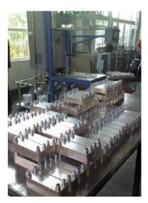
Kaori is currently using the VTech MasSpec for the integral leak detection of their brazed plate heat exchangers. The quality of the leak testing is certified by a calibrated leak and the testing results are recorded to a database for data mining and/or print out of testing certificates.
