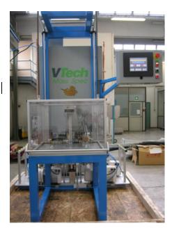
We designed a customized version of conducted the first trials with our VTech MasSpec. This is an automatic helium leak detector, based on outside-in technology. The unit under test is evacuated and exposed to a helium mass spectrometer in a containment chamber filled with a small percentage of helium (between 10 and 20%).
