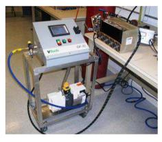
If Pressure Decay is not required or if it is handled by an existing system, then the <u>VTech Gas Fill Plus</u> can be used to evacuate and fill the gas only, and utilize a customersupplied leak detector such as this bench-type configuration with the Gas Fill Plus working alongside the Hydrogen sniffing unit.
