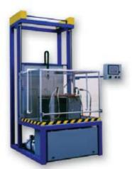
In the VTech CombiTester a U.L. Burst pressure decay test is performed prior to the evacuation, for a complete quality assessment of the units.
